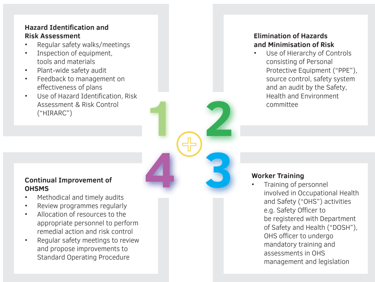
Figure 3: Process of Hazard Identification, Risk Assessment and Improvement of OHSMS
